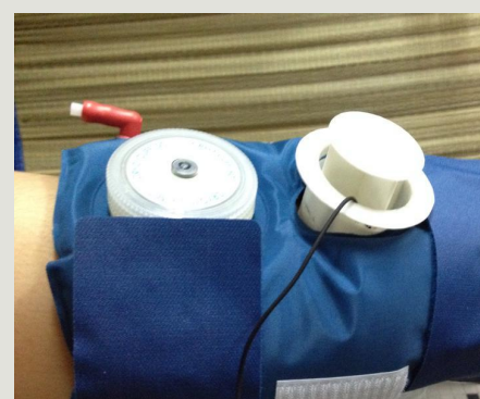
Photo 4: Syringe Knee Pressure Monitor is fit on patient's leg
