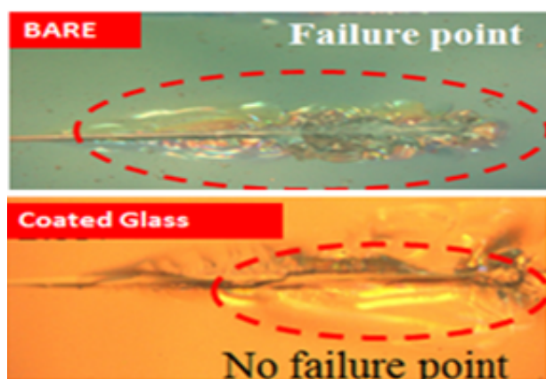
Fig 3: The scratch-resistance of coated glass surface
