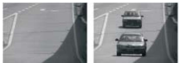
Information from sensors has to be processed before it can be useful to algorithms such as neural networks. Processing information from images consist of several steps. In the figure below the images have to be differentiated from the background before it can be identified as two objects at two different locations.
