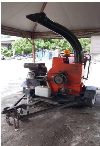
Used to break the compost into smaller pieces
