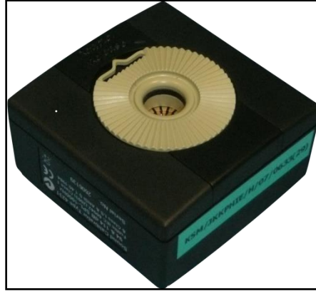
Figure 7.2: Example of sound level calibrator
