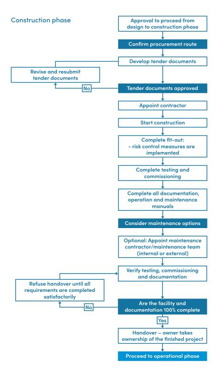
Figure 8.1 Project flowchart, construction phase
